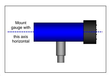
Torr if the unit is not mounted horizontally. Below 1 Torr, mounting position has little to no effect.
