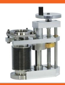
Smooth kinematic linear motion along the port axis (Z) with the additional facility to tilt the travelling flange so it serves as an integrated port aligner. This makes the LSMT ideal for applications where precise alignment with a fixed point is essential.
