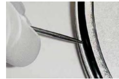
Removal of gate seal
