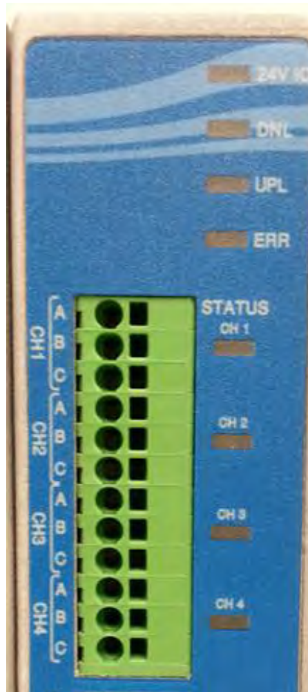
Figure 12- LEDs on Temperature Input module
