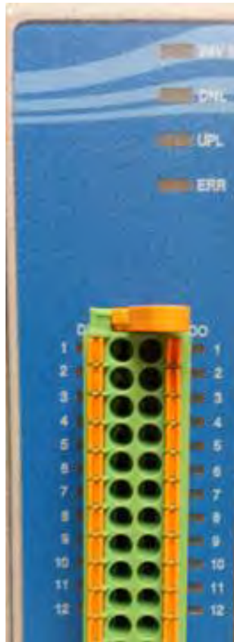
Figure 11- LEDs on PWM Output module
