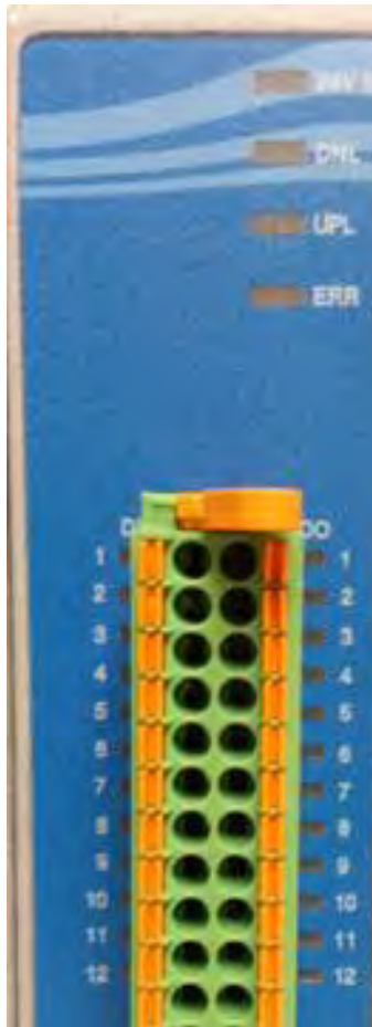
Figure 11- LEDs on PWM Output module
