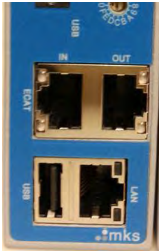
Figure 9- USB, EtherCAT and LAN ports on CPU module
