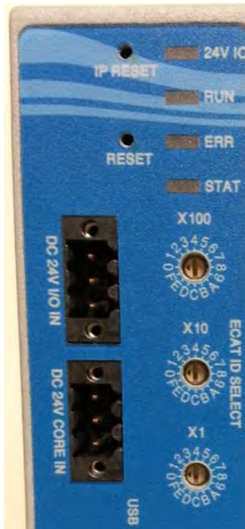
Figure 10- LEDs on CPU module
