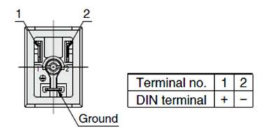
DIN terminal is connected inside as in the figure below.
