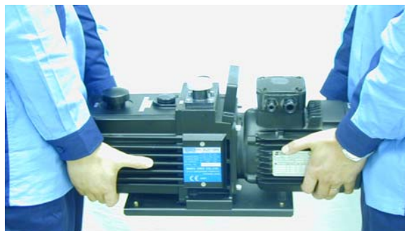
Fig. 3 Transportation method of the oil sealed rotary vacuum pump
