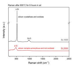
The improved Silcolloy 2000 process allows customers to experience high-temperature stability in their applications. The amorphous silicon layer avoids oxidation at high temperatures to improve and prolong performance.
