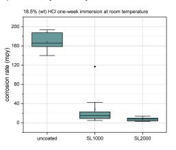
Silcolloy 2000 proves to be the updated standard for corrosion protection, outperforming uncoated stainless steel and its predecessor, Silcolloy 1000.
