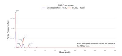
**RGA comparison at 150°C** - No anomalous AMU points on coated samples compared to uncoated, typical expected peaks for  $H_2$ ,  $H_20$ ,  $N_2$ , etc. The difference in peaks between coated and uncoated samples is in the 10e-11 range indicating minimal outgassing differential.
