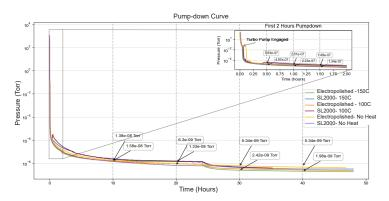
**Pump down comparison at 150°C, 100°C, Room Temp.** - 6"OD CF 304L SS Full nipple test piece coated with SL200 from SilcoTek and compared to uncoated electropolished equivalent. The coated sample enables similar pump down and ultimate vacuum performance to uncoated standards at various temperature levels.
