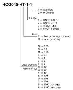
The part number (PN) can be taken from the product nameplate. If not indicated otherwise in the legends, the illustrations in this document correspond to gauges with the DN 16 ISO-KF vacuum connection. They apply to gauges with other vacuum connections by analogy.
