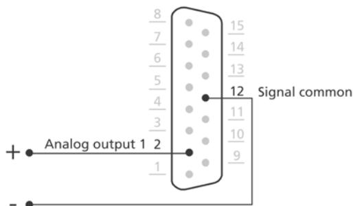
Figure 4-3 Analog output indicating vacuum pressure
