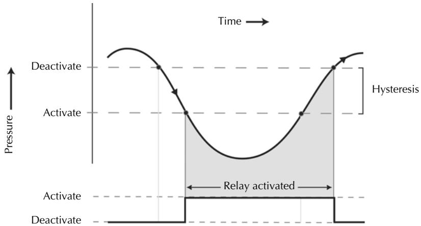
**Figure 5-4** Default behavior of relays activating with increasing pressure ( $A > D$ )
