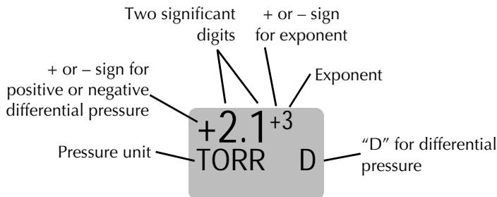
**6.2 Display resolution** Pressure values in the  $10^{-10}$  range (such as  $6 \times 10^{-10}$ ) will appear as “0.6<sup>-9</sup>”. The resolution of the numeric display changes over the operating range of the module. See Table 6-1.
