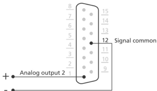
Figure 4-5 Analog output indicating differential pressure
