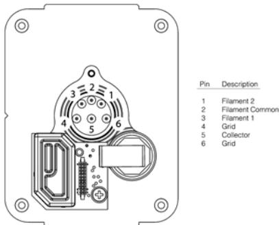
4. Use a digital multimeter to measure the resistance between pins 2 and 3 (the filament pins), and between pins 1 and 2. See Figure 7-2. The readings should be  $0.2 \Omega$ .
