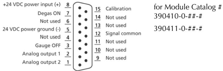
**Figure 2-3 Wiring terminals for Micro-Ion ATM module with RS-485 interface, two analog outputs, and no trip-point relays**
