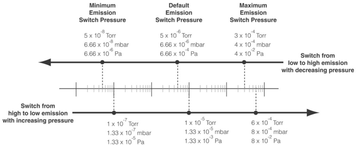
Use the set emission range (SER) command to set or read the pressure at which the Micro-Ion gauge switches from low to high emission current with decreasing pressure.
