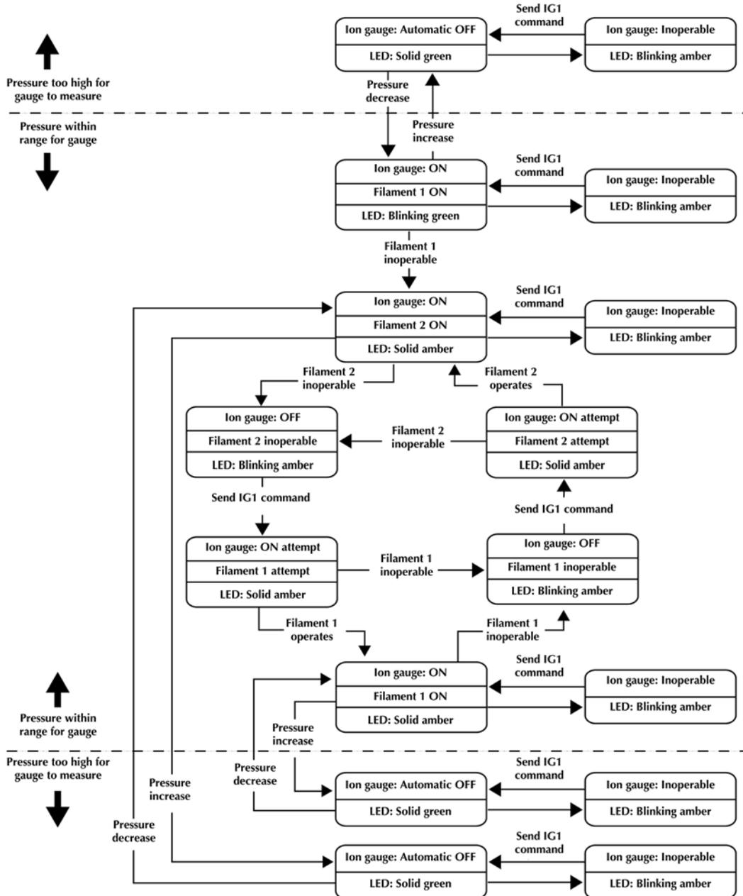
NOTE: The Micro-Ion Module is factory configured for either single-filament or both-filament operation at low emission.
