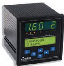
The PDR900 power supply and readout unit is a stand alone, single channel controller for use with the Series 900 digital vacuum transducers. It can be used as a stand-alone power supply readout unit or as a tool for configuration, calibration and diagnostics of system integrated transducers in OEM applications.
