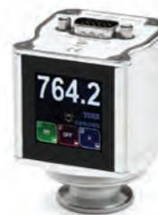
The optional integrated touch-screen display is user configurable; the user can change pressure units, orientation and has access to set point parameters as well as gas type. The display also indicates the status of the available set point relays. Displayed reading can be seen from >5 meters away on the high contrast display.
