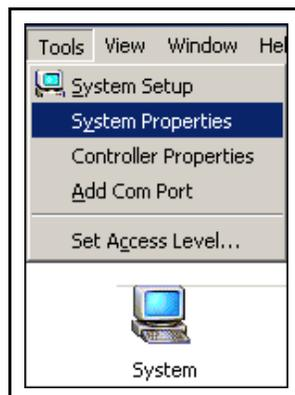
The first time the XTC/3 Editor is run it starts on the **System Setup Screen** and prompts for a communications port (Com Port) to be configured. See [Figure 2-2](#). From this dialog, select and add the Com Port to be used for communications with the XTC/3 Thin Film Controllers.
