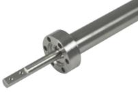
Unguided linear motion solutions for low load applications in high/ultra-high vacuum. The vacuum shaft is free to rotate, avoiding possible conflict with an internal chamber mechanism. Available in CF16 and CF35 flanges and six stroke lengths from 50mm to 300mm. Manual, pneumatic and motorised actuation options with additional switches to prevent over-travel.
