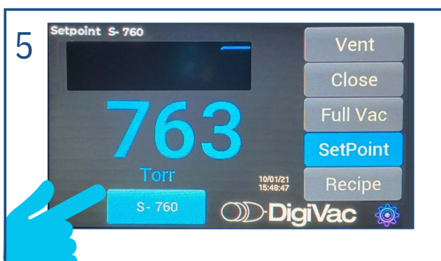
5 Select Set point as shown (or other options such as Mode or Recipe and play)
