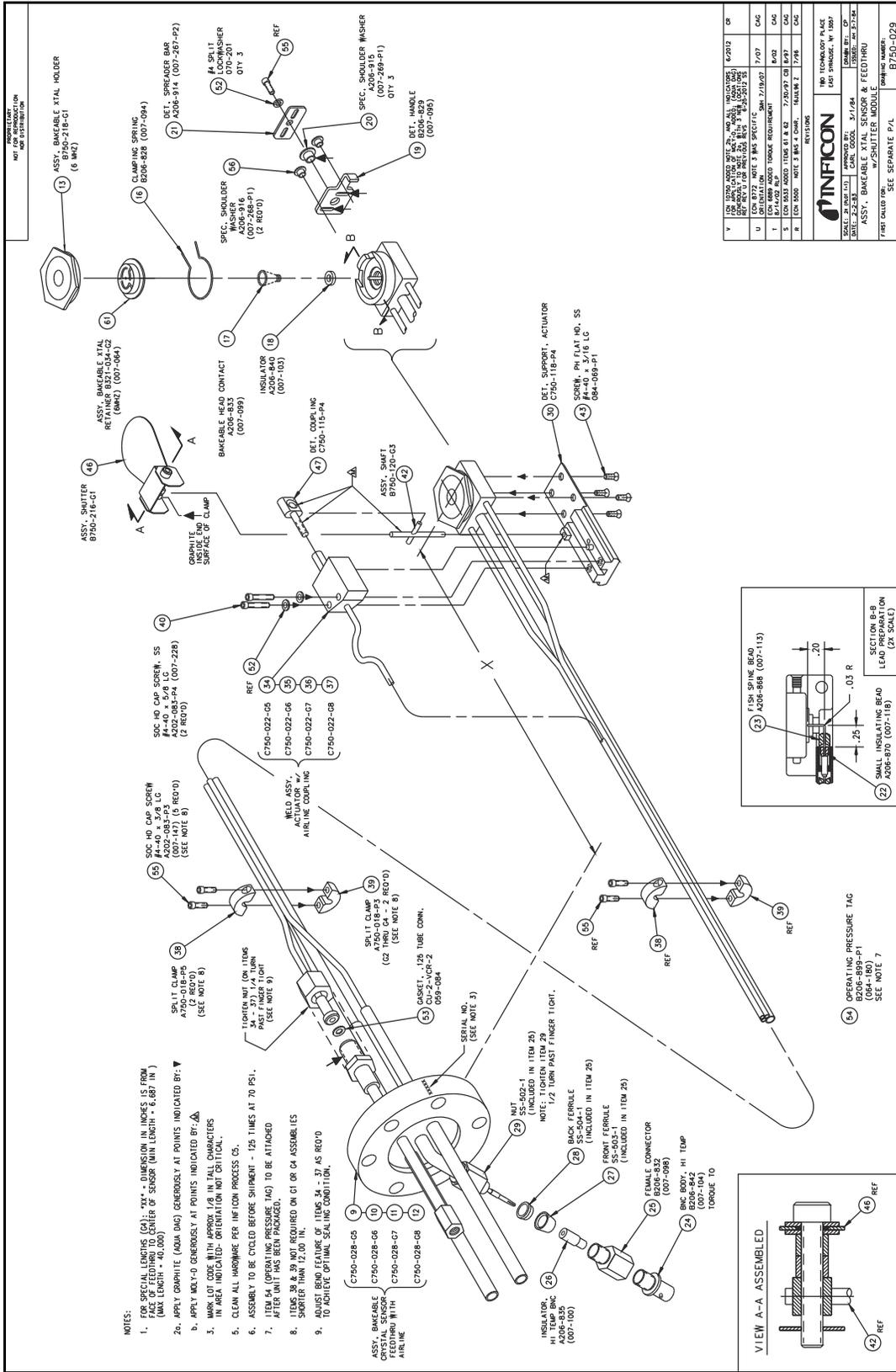
Figure 1-7 Shuttered UHV Bakeable Sensor with feedthrough assembly
