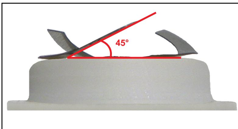
To adjust the prongs on the leaf spring positioned on the ceramic retainer, touch the end of the prong with a gloved finger, or grip the prong with Teflon tweezers, and gently lift it upward. Be careful not to kink the prongs. An ideal bend has a smooth, sweeping shape (see [Figure 4-3](#)).
