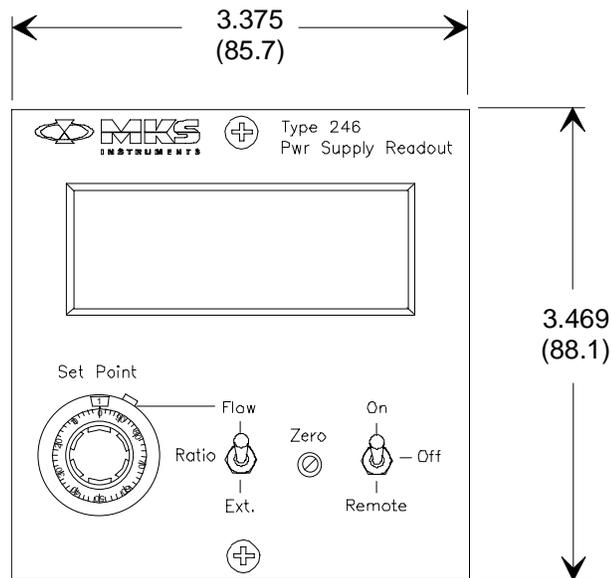
Figure 1: Front Panel Dimensions
