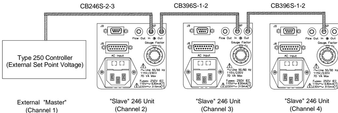
Figure 6: External Set Point Control Setup - Ratio Flow Control
