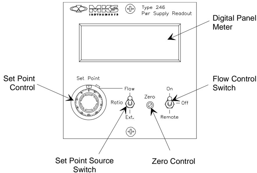
Figure 7: Front Panel Controls
