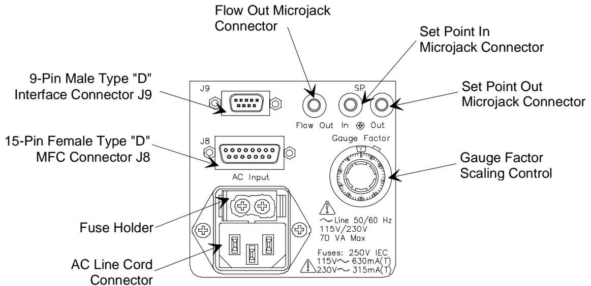
Figure 8: Rear Panel Controls
