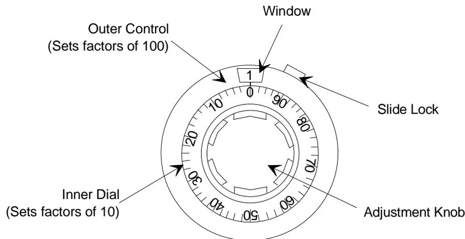
Figure 9: Scaling Control Potentiometer - Initial Setting
