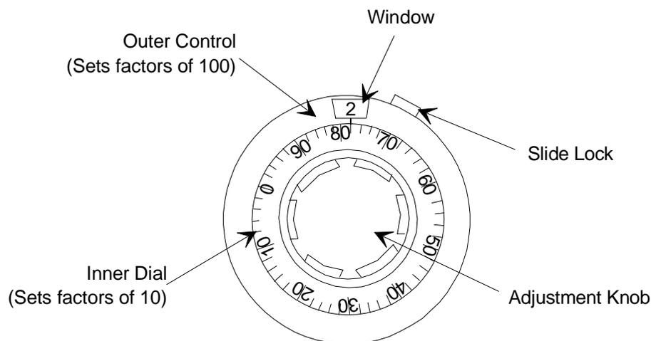
Figure 11: Gauge Factor Scaling Control Potentiometer - Example Setting
