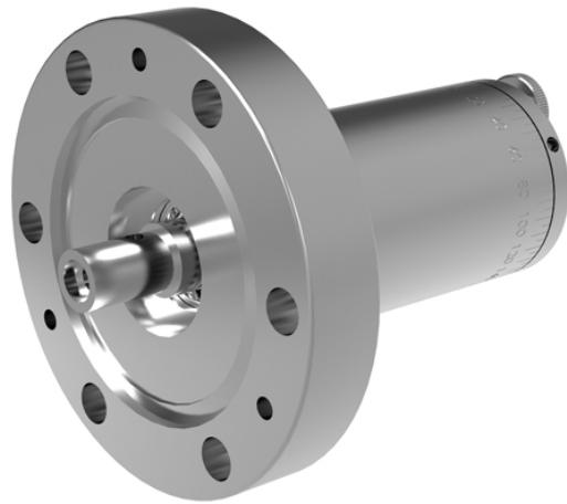
The MD40N MagiDrive provides low torque rotation (0.45Nm) on a 70mm OD (2 $\frac{3}{4}$ " OD CF) flange. The MD40A MagiDrive provides medium torque rotation (1.8Nm). The drive is ideally suited to applications such as the rotation of samples and small platens, where stability is key.
