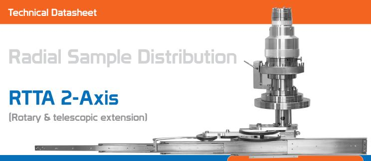
The 2-axis RTTA provides 360° rotation and 760mm linear extension within an ultra-compact footprint. Less than 1mm deflection at full arm extension with 10N load, linear reproducibility of <0.1mm and rotational reproducibility of <0.2mRad. Motorization options available.
