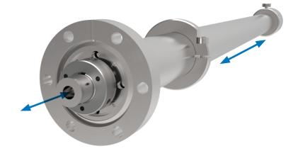
High performance magnetically-coupled linear devices, designed for sample transfer where only linear motion is required and rotation is undesirable. Available in standard stroke lengths from 304mm to 1524mm with motorisation options. The LPP is bakeable to 250°C without removing any components.
