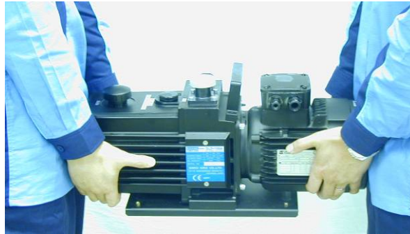
Fig. 2 Transportation method of the oil sealed rotary vacuum pump
