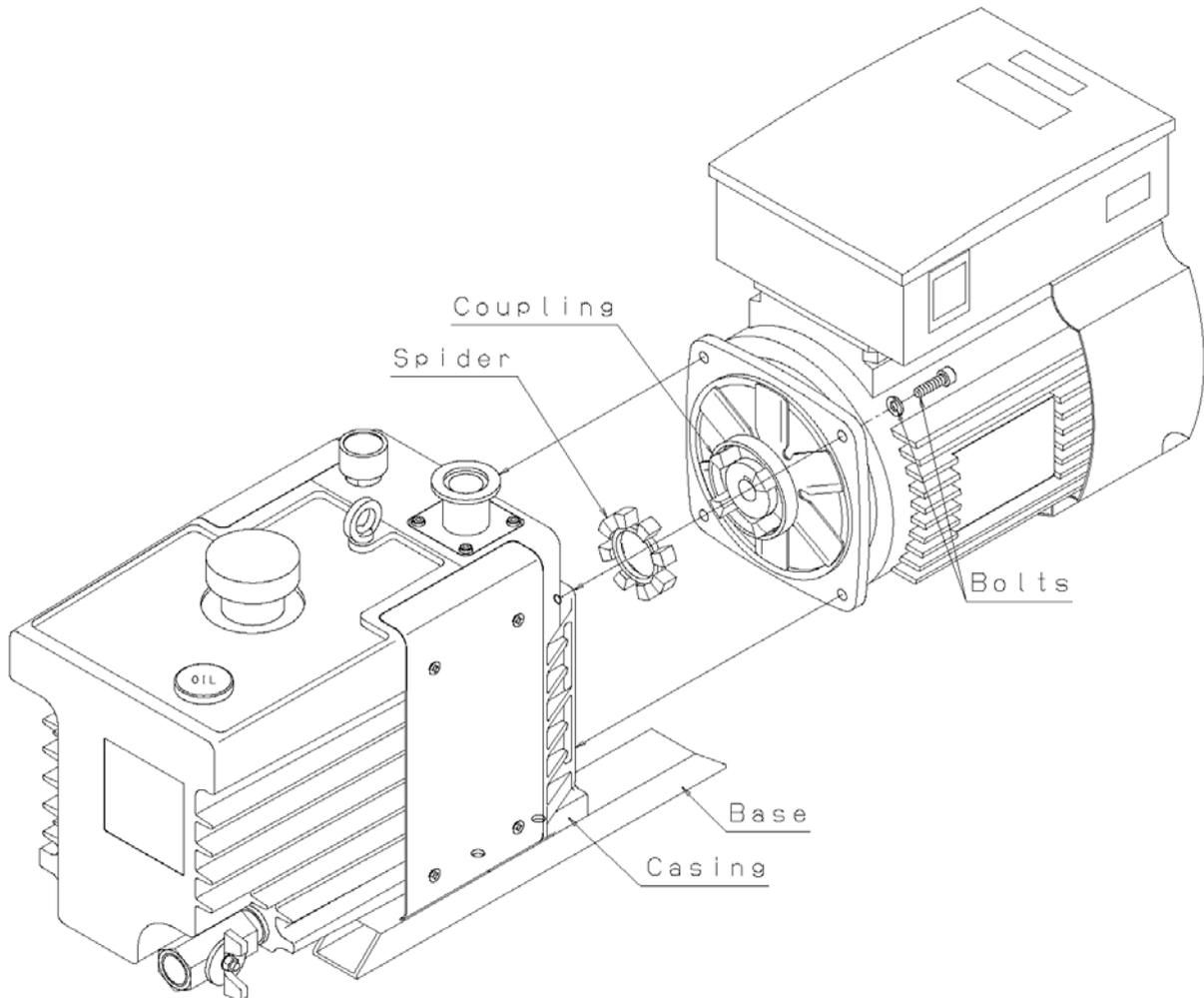
Fig. 10 Replacement of the coupling spider
