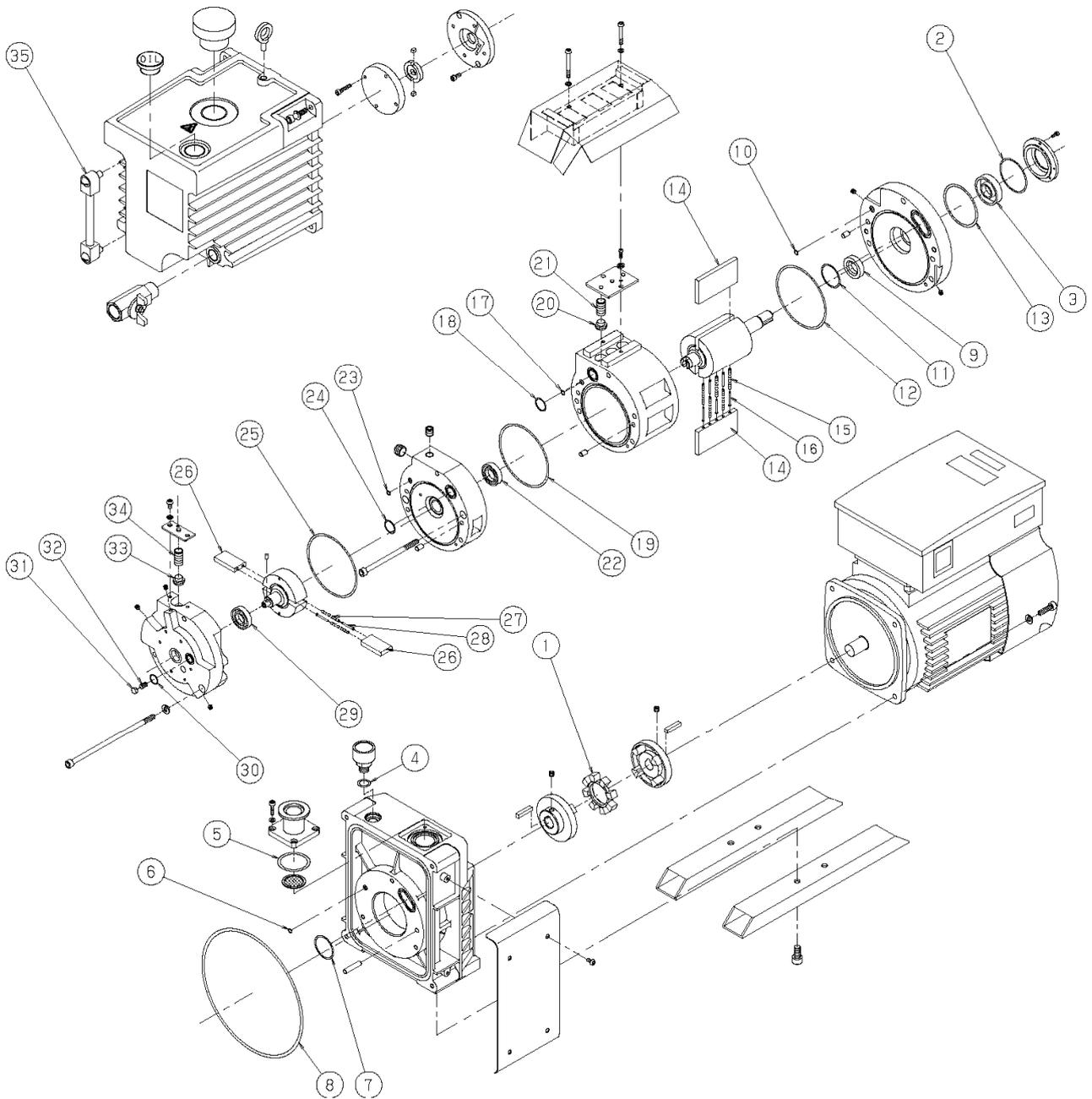
Fig. 11 Disassembly drawing of GLD-280B oil sealed rotary vacuum pump
