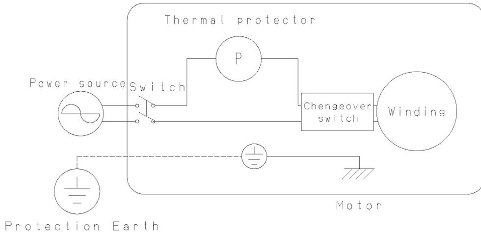
Fig. 5 Electric wiring diagram
