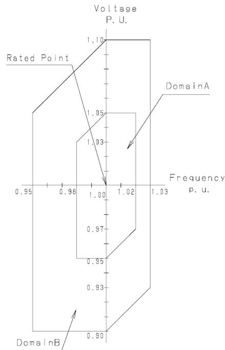
Fig. 8 Change region of the voltage and frequency
