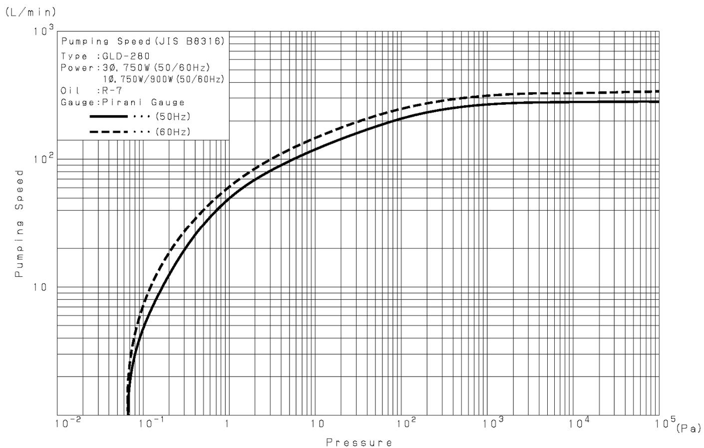
Fig. 9 Pumping speed curve
