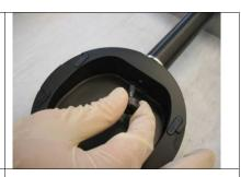
Remove the valve gate from the valve insert assembly. Pull down the bellows feed through unit from the actuator shaft and exchange this part with a new one.
