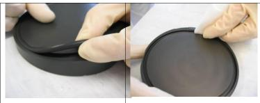
Remove the gate gliders from the valve gate with a little tool e.g. screwdriver.
