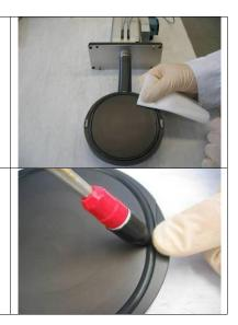
Remove the o-ring from the groove and clean the groove with alcohol.
