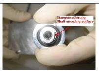
Move the new bellows feedthrough unit on the actuator shaft until you can see the flat encoding sections for the valve gate, followed by the assemble of the o-ring onto the bellows feedthrough.
