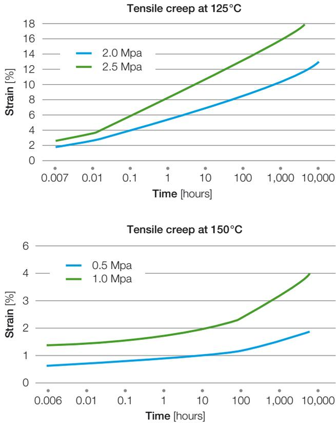
Stress relaxation is defined as the reduction in strain needed to maintain a constant stress. This physical phenomenon is a uniquely measured form of creep.
