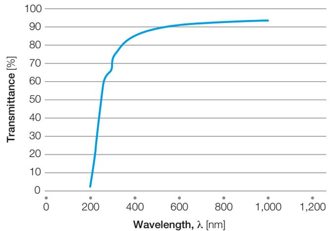
**Figure 11:** ATR-IT (attenuated total reflection-infrared) spectrum of Halar® ECTFE 500 thin film (transmission).
