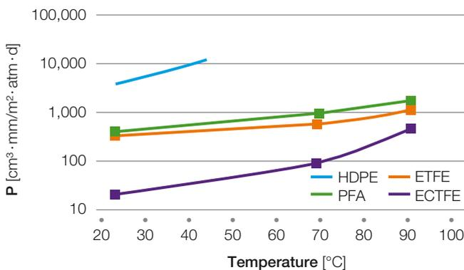
**Figure 30:** Hydrogen sulfide permeability of Halar® ECTFE compared to other polymers
