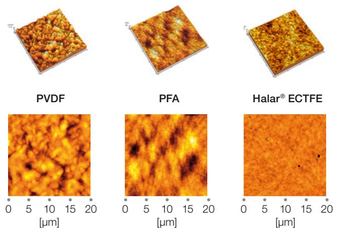
Furthermore, as shown in Figure 9, Halar<sup>®</sup> ECTFE pipes exhibit a low incidence of microbial bio-fouling, making it ideal to use in ultrapure water (UPW) applications.
