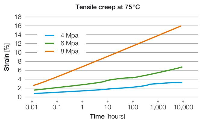
**Figures 19 and 20:** Tensile creep of Halar® ECTFE at various temperatures and under different stresses
