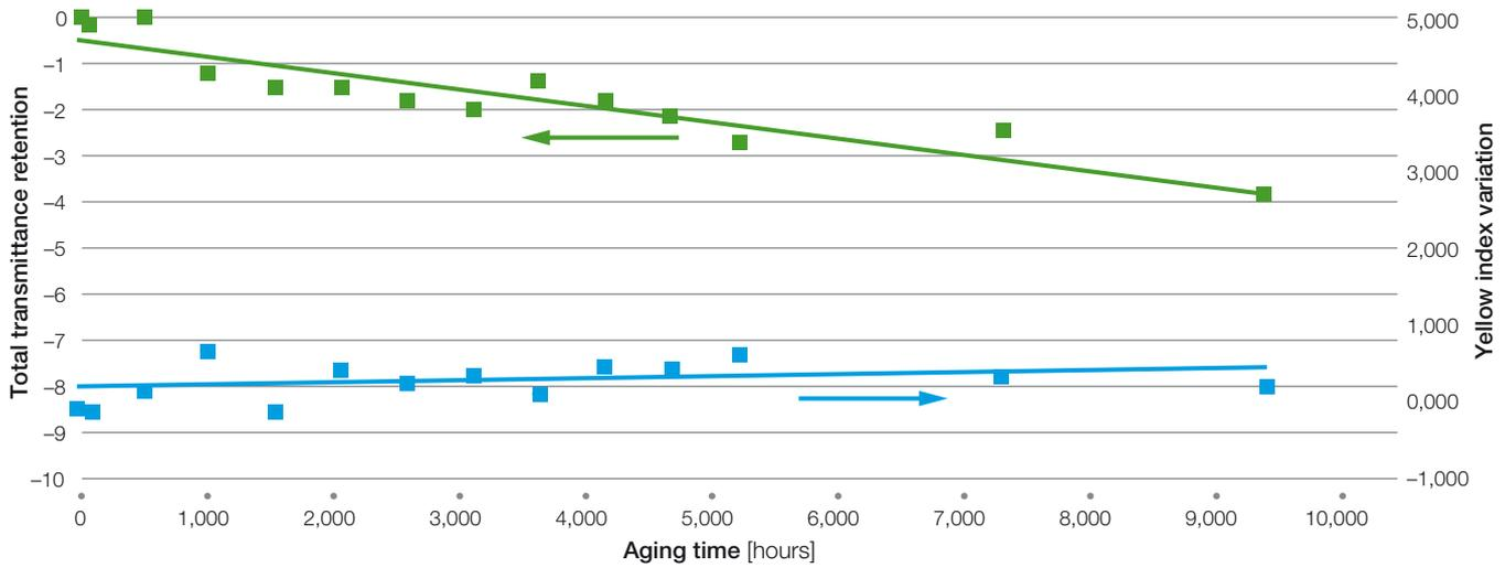
**Figure 36:** Optical properties of Halar® ECTFE films under 10,000 hours of Xenon Arc weatherometer
