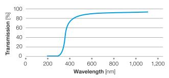
This feature helps to protect EVA and other encapsulants from degradation in photovoltaic modules if used as frontsheet or transparent backsheet and prevents PET degradation in both photovoltaic structures (plus any other outdoor use) and in all potential plastic composites exposed to sunlight.
